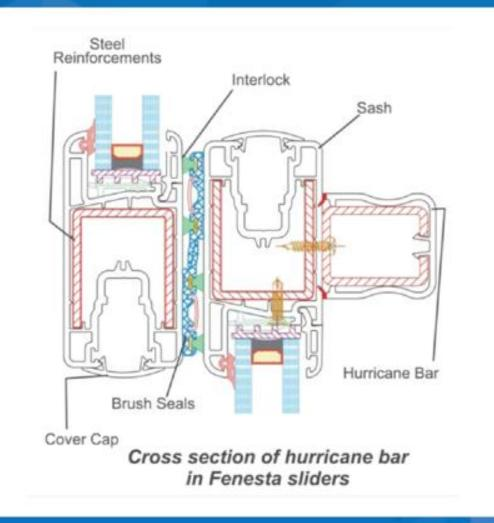
Hurricane Bar can Withstand Wind Speeds up to 245kmph
