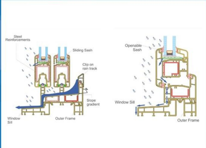
Special Rain Track & Sill Arrangement to block rain water seepage
